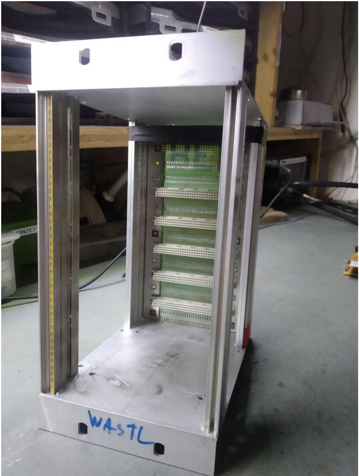
Figure 9: The case with installed backplane
